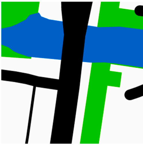
Fig. 1. A customised roadmap image (map type: road map, size: 256 \times 256 , zoom level: 19) defined the background as white, roads as black, water as blue, and parks as green.
